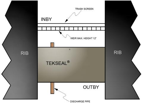
If a new seal is placed on the outby side of an existing seal equipped with a water drainage system, the existing U-trap must be removed, the existing valve must be removed or placed in a fully-open position, and the drainage pipes must be extended through the new seal with a new valve and U-trap installed as required and meeting required specifications discussed in this section.
